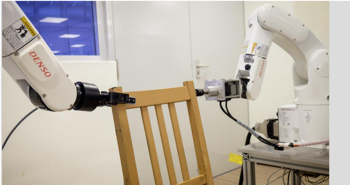
Robot assembles IKEA's Stefan chair. Photo: NTU Singapore
